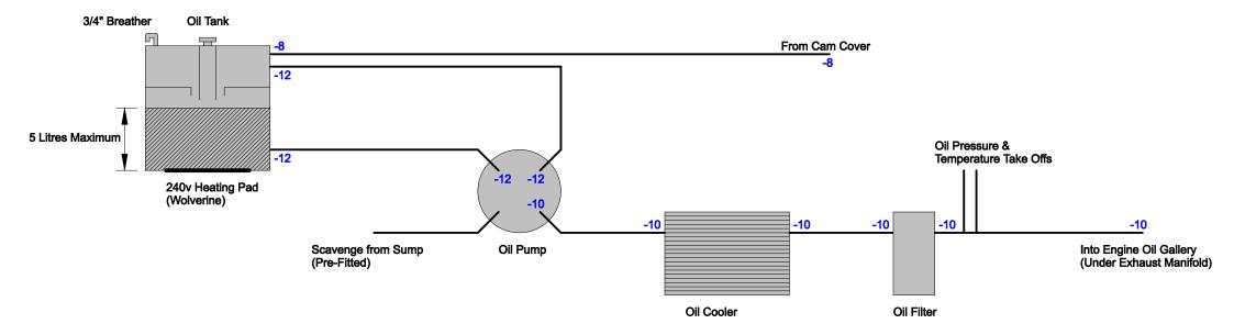
All pipes and connections to to be absolute minimum bore size of 13mm.
